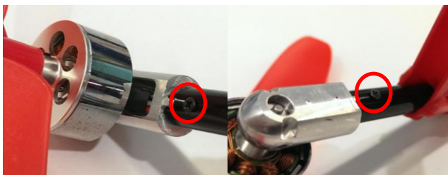
Step 6: Apply the short screws to the point that connects the motor arm and the mount
